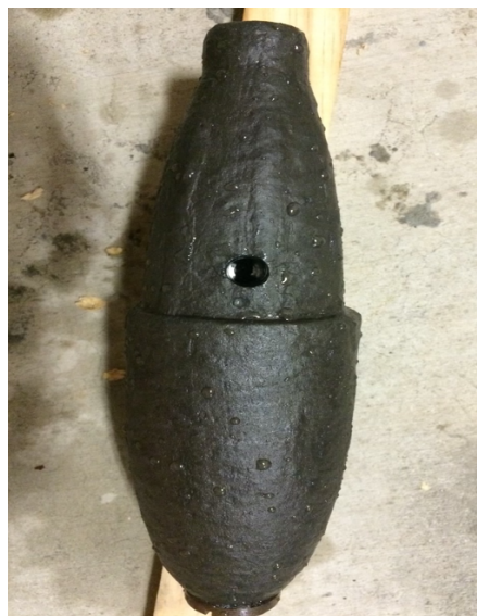
Fig. 8. Schenkl Shell with brass impact fuze intact.
